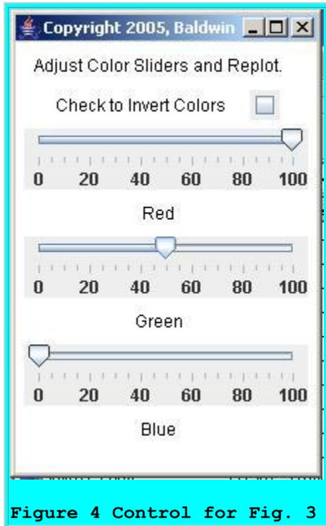
The red slider in Figure 4 is positioned at 100, causing the red color values of all the pixels to remain unchanged. The green slider is positioned at 50, causing the green color values of all the pixels to be reduced to 50% of their original values. The blue slider is positioned at 0 causing the blue color values of all pixels to be reduced to 0.
